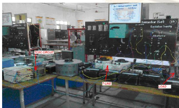
Fig.8 Lab setup of SMTB system with TCSC
