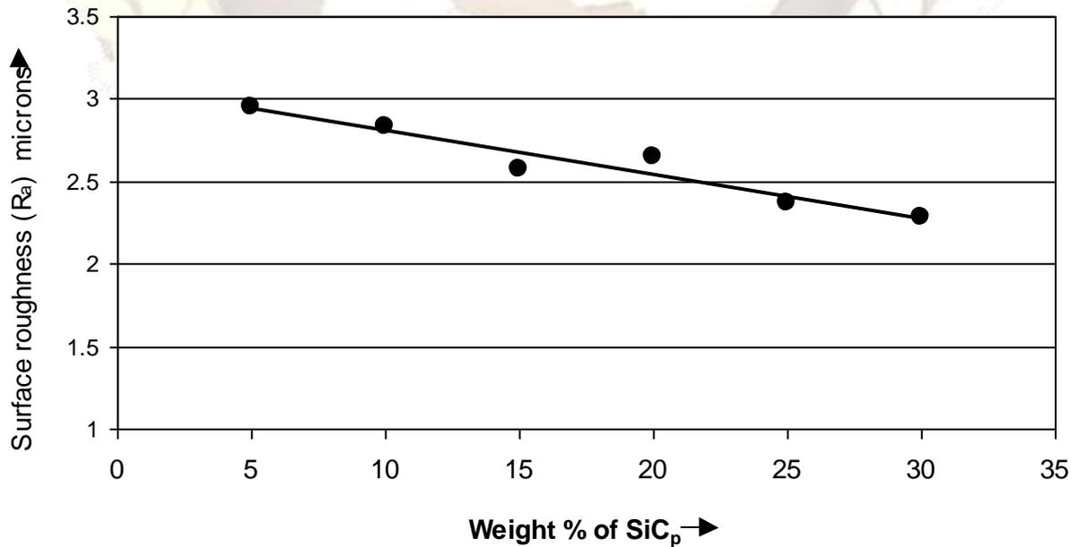
Fig. 13 Surface roughness of PM Al-SiC<sub>p</sub> composites
