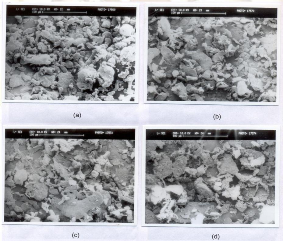
Fig. 5 Scanning electron micrographs of the Al powders with 10 weight % of SiC particulates (a) before ball milling, irregular particles; (b) after 4 hours of ball milling, flat lamella structure; (c) after 8 hours of ball milling cluster type structure and (d) after 12 hours of ball milling, equiaxed. (Mag. X400)
