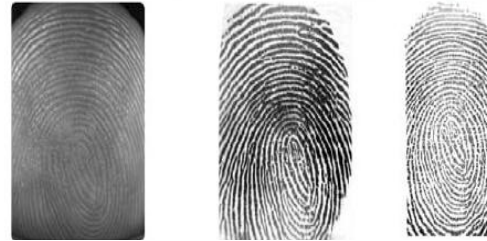
Fig.3.Fingerprint image using optical sensor/Line sensor
