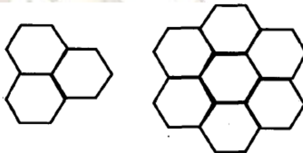
Fig2 : Illustration of cell cluster N=3 & N=7
