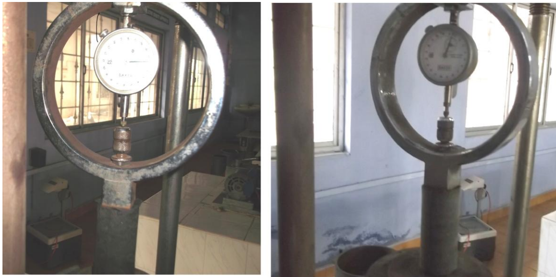
Fig.3 Unconfined Compressive Strength test on soil with Bitumen Emulsion and Sea Shell Powder
