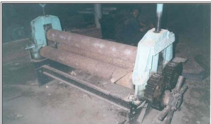
Fig.1: Manually operated Sheet Bending Machine Showing Spur Gears and Handle Arrangement
