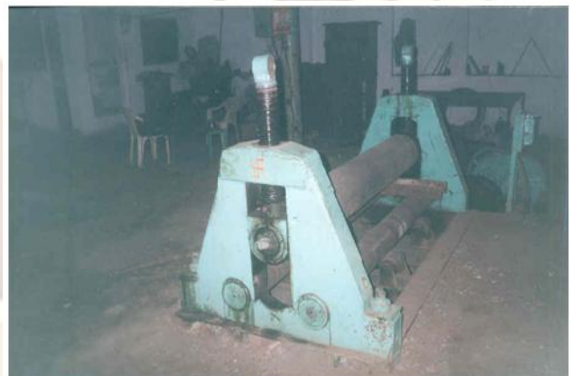
Fig.2: Power Operated Bending Machine Showing Roller and Adjustable Screw Arrangement
