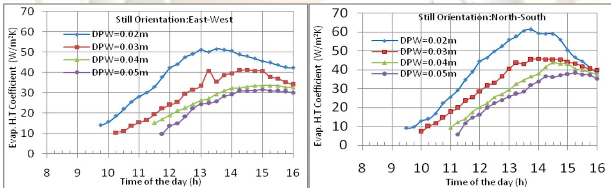
**Fig.4.3. Variation in evaporative heat transfer coefficient**
