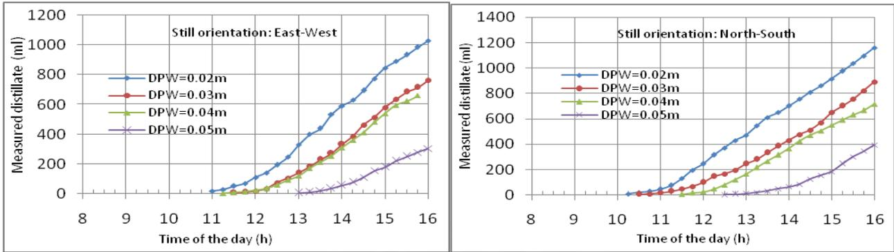
Fig.4.4. Variation in the measured distillate output
