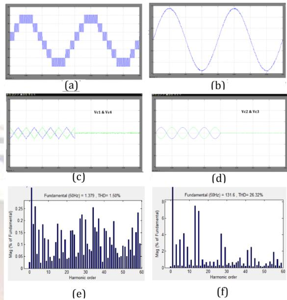
Fig-10 (a)Phase Voltage & (b)Current waveforms for the four-level operation
