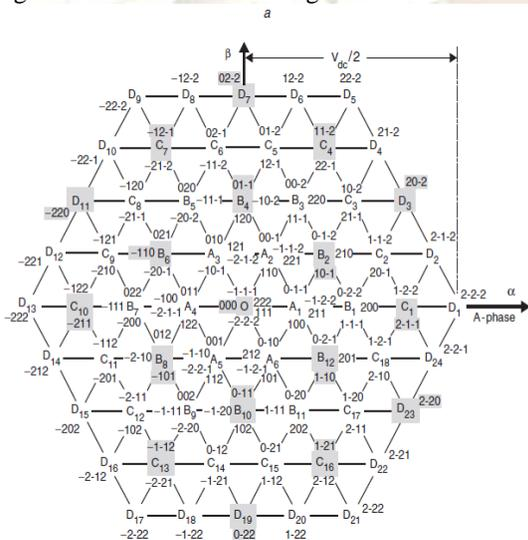
Fig : 2 Switching states and voltage space vector locations of five-level inverter (A or A')
