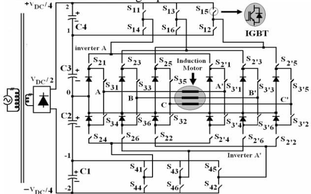
Figure 1. Power circuit of the five-level inverter for open-end winding induction motor drive.
