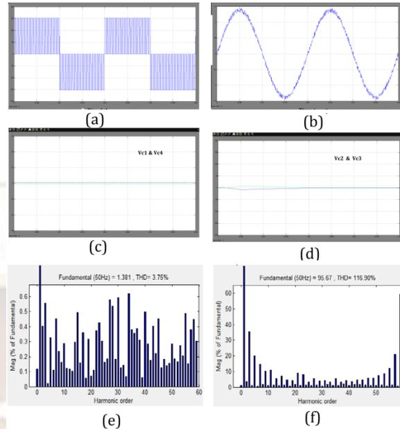
Fig-8 (a)Phase Voltage & (b)Current waveforms for the two-level operation (c) & (d) Variation of capacitor voltages during disabling and enabling of control (e) & (f) Spectra of the phase current and phase voltage.
