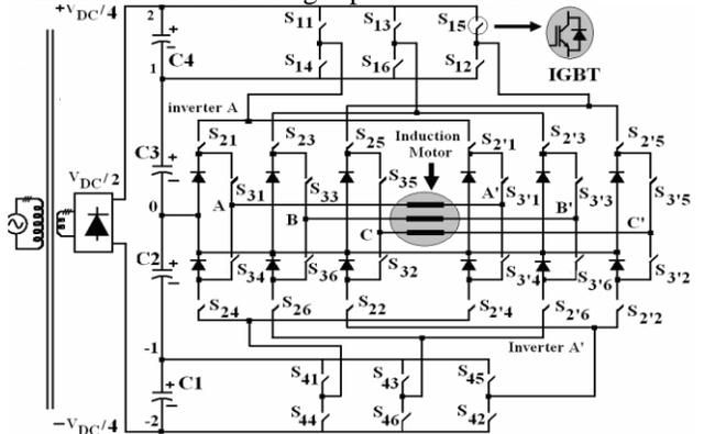
Figure 1. Power circuit of the five-level inverter for open-end winding induction motor drive.
