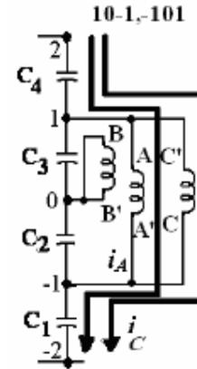
Fig.-5: Connection for the switching state of the voltage vector at  $B_1$ .
