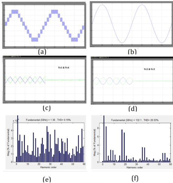
Fig-11 (a)Phase Voltage & (b)Current waveforms for the four-level operation (c) & (d) Variation of capacitor voltages during disabling and enabling of control (e) & (f) Spectra of the phase current and phase voltage.
