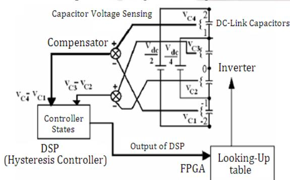
Fig.-7: Hysteresis controller for the closed-loop control of the dc-link capacitor voltage balancing
