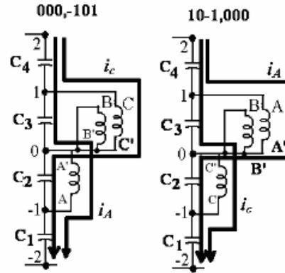
Fig-3 Connection of the three phases for the two switching states at  $A_1$
