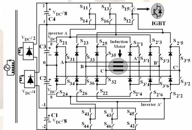
Fig-4. Modified circuit diagram of the five-level inverter-fed IM drive
