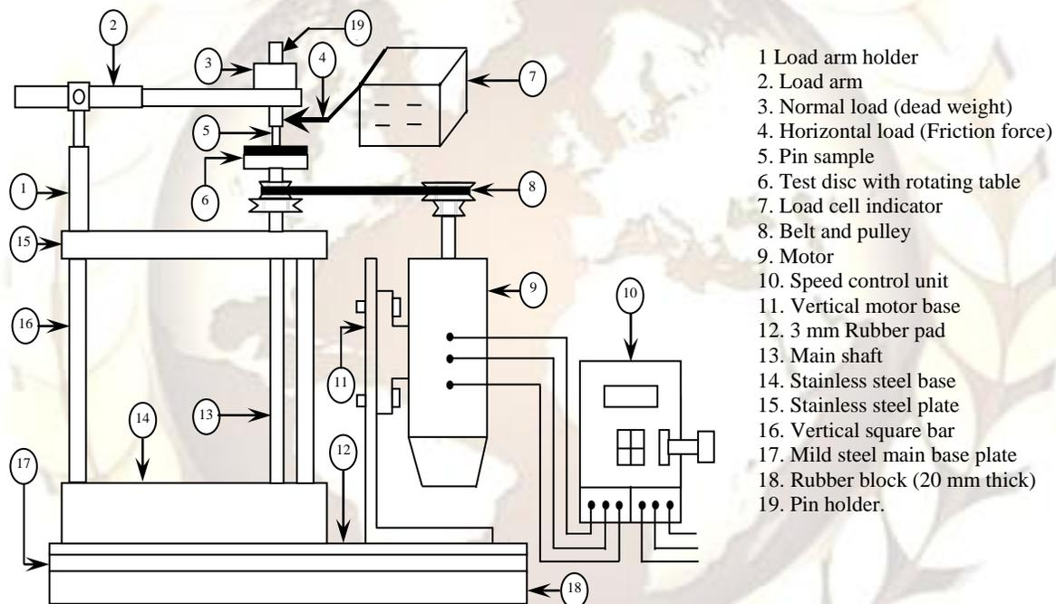
Fig. 1 Block diagram of the experimental set-up
