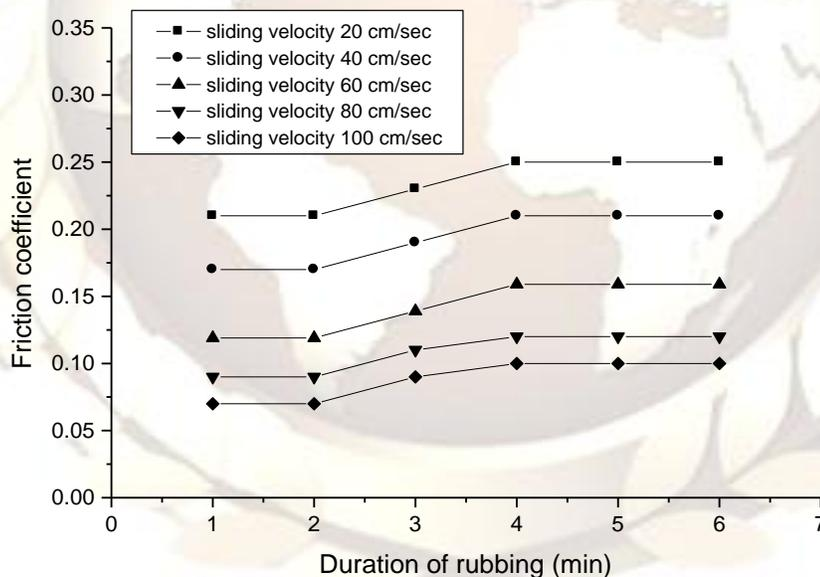
Fig. 3: Variation of friction coefficient with the variation of duration of rubbing at different sliding velocity for brass-MS pair (Normal load=10 N, Relative humidity=80%)
