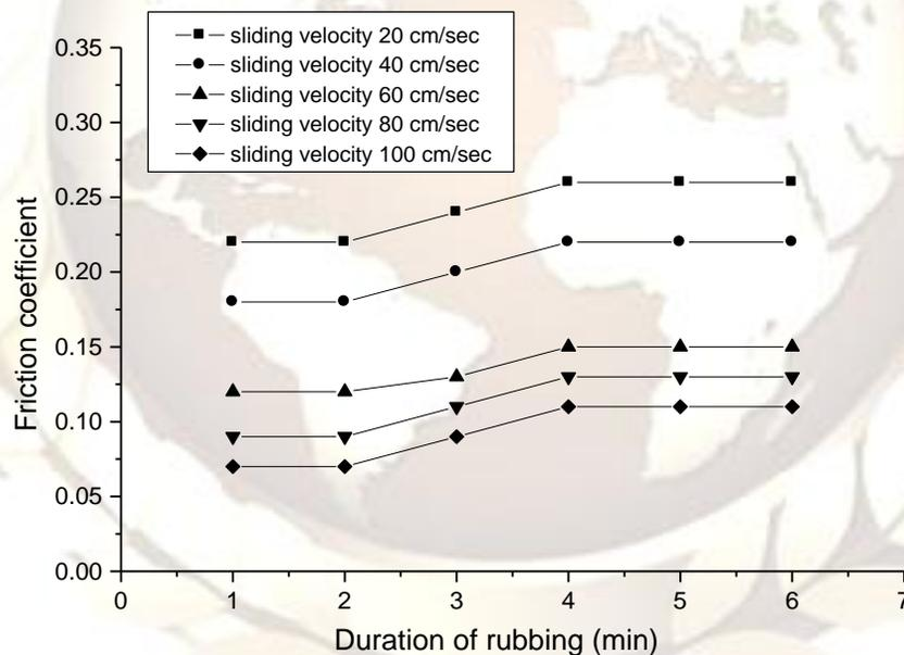
Fig. 5: Variation of friction coefficient with the variation of duration of rubbing at different sliding velocity for brass-SS pair (Normal load=10 N, Relative humidity=80%)
