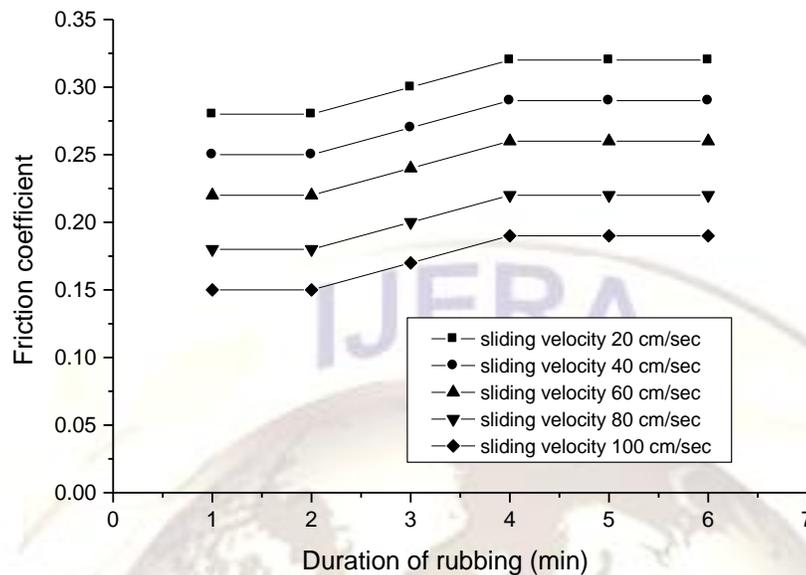
Fig. 4: Variation of friction coefficient with the variation of duration of rubbing at different sliding velocity for brass-SS pair (Normal load=10 N, Relative humidity=60%)
