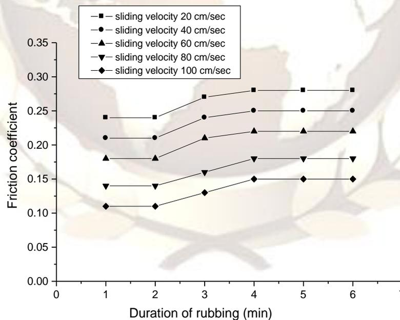
Fig. 2: Variation of friction coefficient with the variation of duration of rubbing at different sliding velocity for brass-MS pair (Normal load=10 N, Relative humidity=60%)
