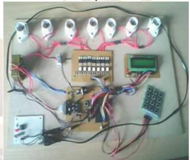
Figure 3: Diagram of Main Project Kit Microcontroller: Microcontroller being the main module has home appliances control system installed on it. Appliances control is responsible for ubiquitous access of appliances. Systems work on GSM technology for transmission of instructions from sender to receiver.
