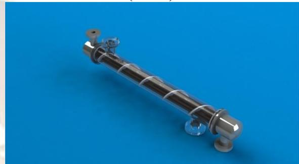
**Fig.2 Shell and tube Heat Exchanger with continuous Helical Baffle (STHXHB)**
