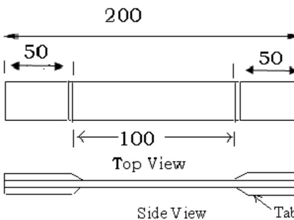
Fig.3. Sketch of lamina Specimens with tab.
