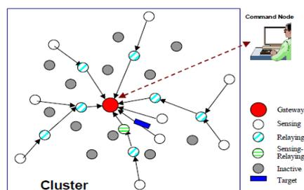
Figure 8.A Typical Cluster in a Sensor Network
