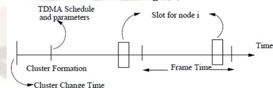
Figure 7. Time Line for APTEEN
