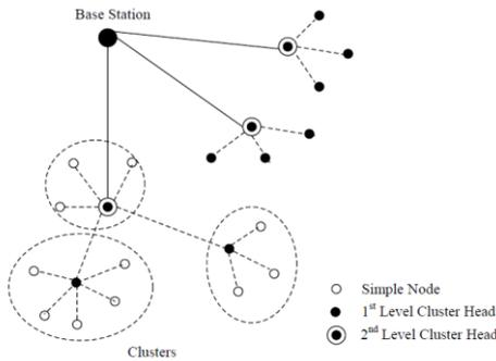
Figure 2. Cluster-based Hierarchical Model
