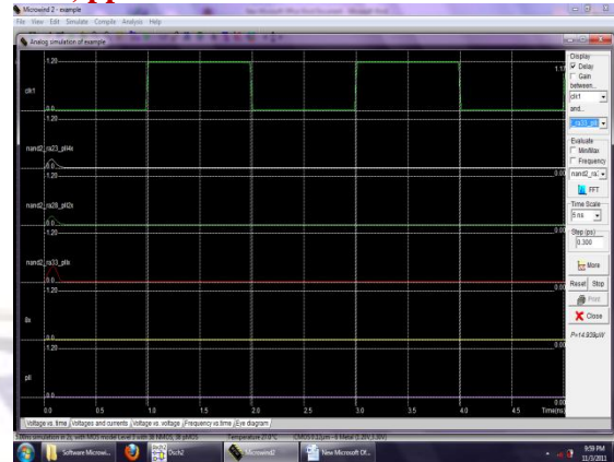
Fig 10 voltage vs time response of proposed pll The PLL is locked at 3.3 GHz frequency. Figure-8 shows voltage versus time waveforms of PLL's outputs and inputs. When control voltage is reaches to 0.415 volt, PLL is locked to the frequency of 1.3 GHz. Multiple output of the PLL gives multiple frequencies of amplitude 1 volt.
