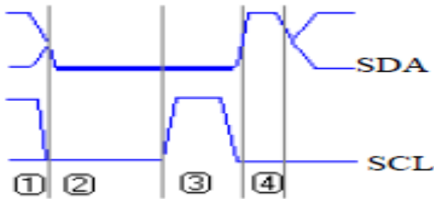
Fig. 7. Clock polarities with SDA and SCL
