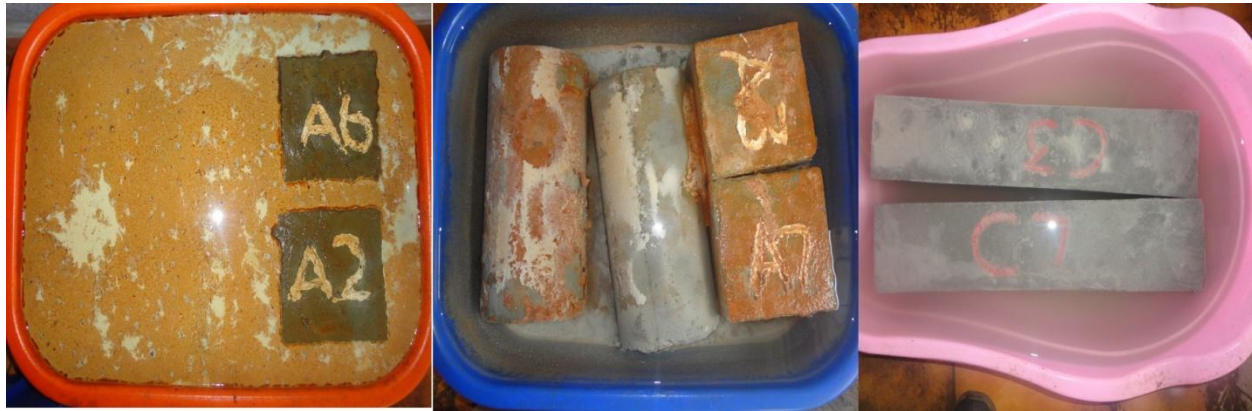
Figure 2 Curing of specimens in effluents 1, 2 and 3.
