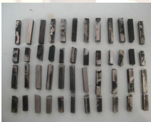
Fig. 7, Broken specimens after impact test specimens
