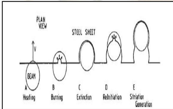
**Fig:1 Schematic mechanism of formation of striations during laser cutting**
