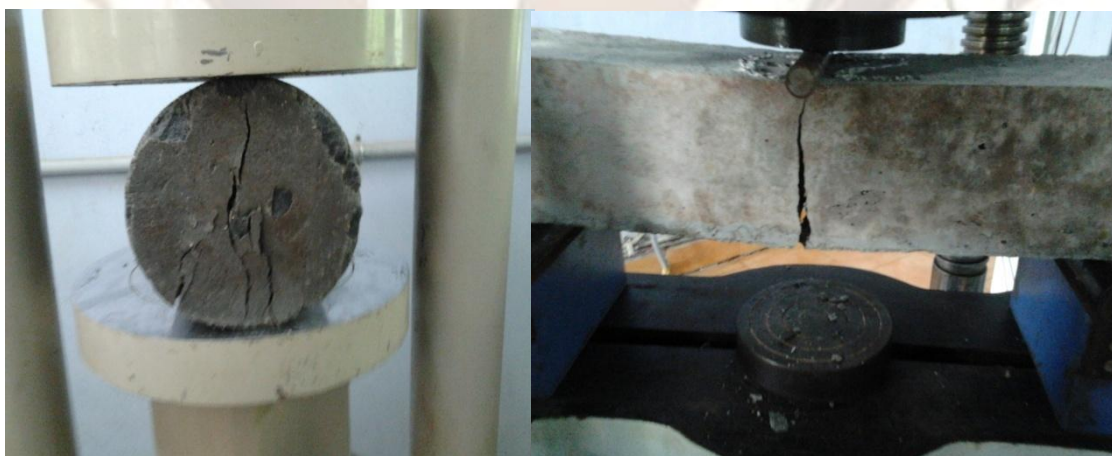
Fig 5: Split tensile and flexural failure of concrete
