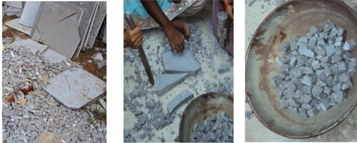
Fig 1: Shabath Stone Source, Manual Cutting and Preparation of Aggregate
