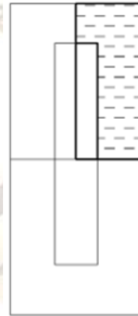
Fig 2: Complete model of fiber and matrix in unit cell
