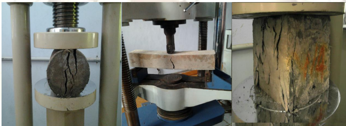
Fig 5: Failure Modes of Specimens
