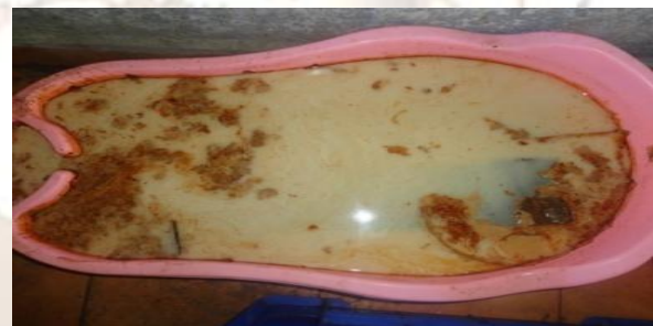
Fig.4 Curing of specimens in E1
