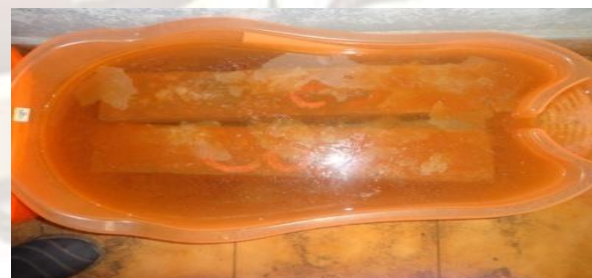
Fig.5 Curing of specimens in E2
