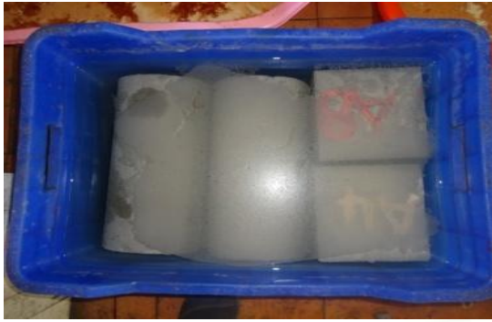
Fig.6 Curing of specimens in E3
