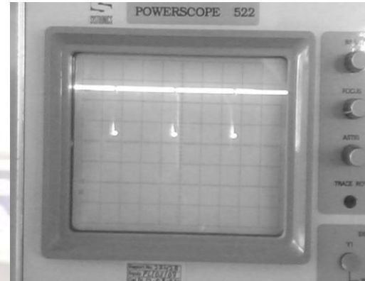
Figure 4 Waveform of PWM ckt. at MAX. pot position
