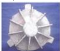
Figure 2.1.5: Al Casting Developed Using FDM Pattern
