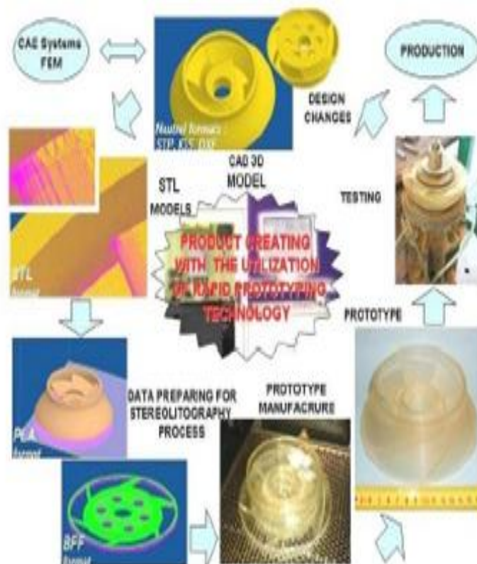
Figure 3.2.1: Cycle of the integrated Product Development of the Pump Rotor with the Utilization of Stereolithography Technology (SLA) An iterative process of product development in north Poland Company occurs when errors are discovered or more efficient, better design solution are looked for study of an earlier generation prototype of pump rotors .Traditionally, the main problem involves a series of advanced machining processor utilizing a variety of expansive tooling; it is time consuming & cost consuming. Manufacturing take several months to prepare and the production of a single complicated part, as a pump rotor, by conventional machining operation can be very difficult. Those factors were the main reasons to utilize stereolithography technology for pump rotor manufacturing at Gdansk University of Technology.
