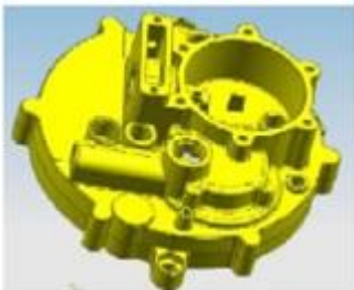
Figure 4.3.2: CAD Model of the Part was Developed with aid of 3D Digitizing Machine
