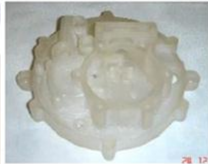
Figure 4.3.4: Rapid prototyping model was developed using Invision 3D printer. This model will be used to re-produce the optimized part with the new dimensions and modified details through the Investment casting techniques.
