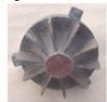
Figure 2.1.1: Original wooden pattern
