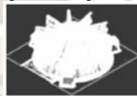
Figure 2.1.2: Laser Scan CoPs Data Using Renishaw Cyclone Scanner
