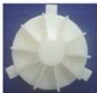
Figure 2.1.4: FDM Plastic Pattern
