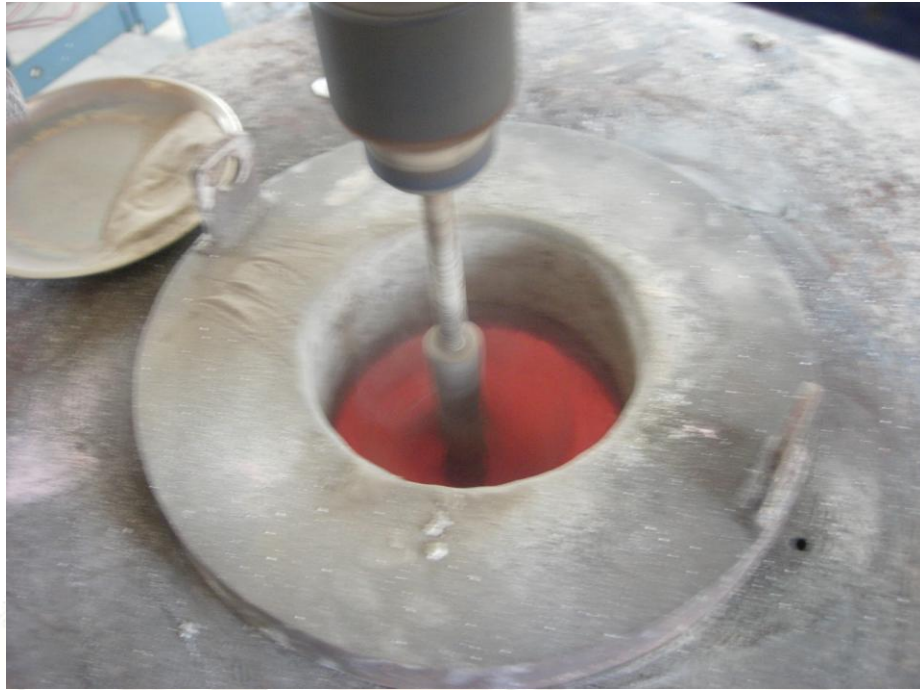
Figure1: Close-up view of stir-casting set-up. \text{Al}_2\text{O}_3 particulates of various sizes are added to the melt at 730^\circ\text{C} which is continuously stirred using a motorized ceramic coated stainless steel rod.
