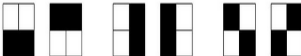
Horizontal Shares Vertical Shares Diagonal Shares Fig. 2 Pixel encoding in (2, 2) Visual Cryptography scheme
