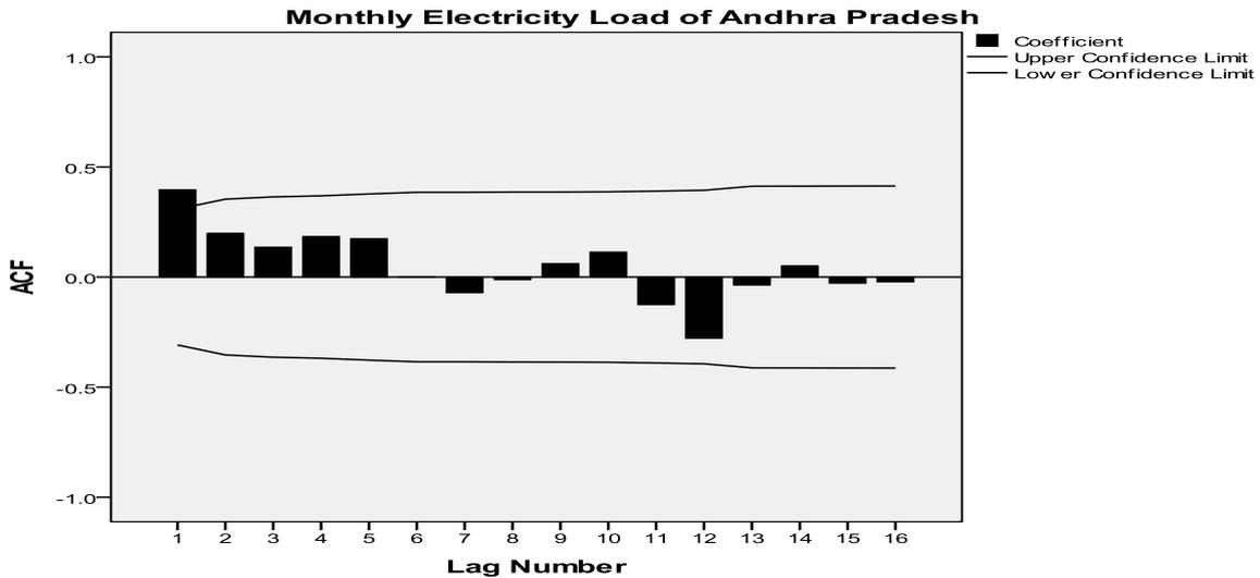
Figure 4. Sample ACF with with  $d=1$ ,  $D=1$  and period 12.
