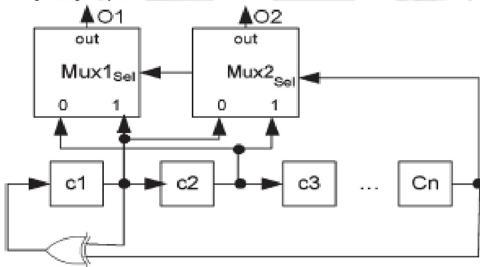
Fig2: External LFSR that implements proposed swapping arrangement.
