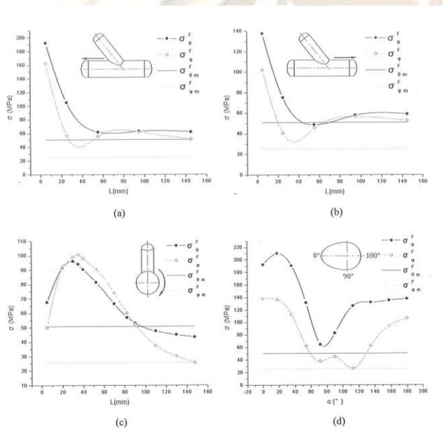
Fig. 5 FEM stress distributions for model 1 ( $\theta = 60 \text{ deg}$ )
