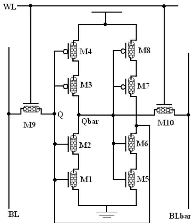
Fig. 4: The Proposed Forced Stack CNTFET SRAM Cell
