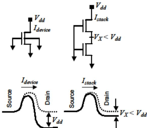
Fig. 3: Leakage current difference between a single OFF device and a stack of two OFF devices.
