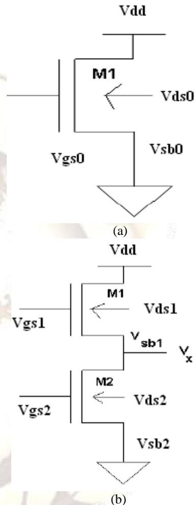
Fig. 2: (a) Single Transistor (b) Forced Stack Transistor
