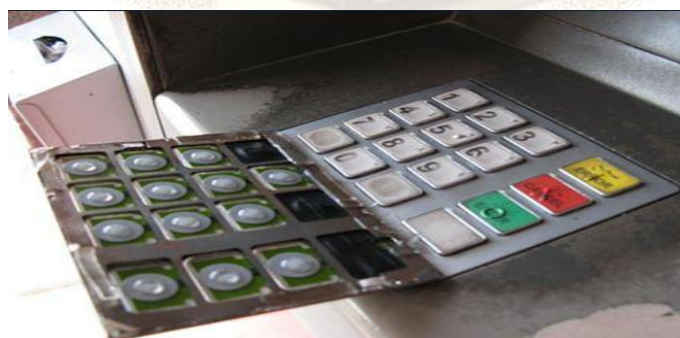
Figure 1.1: Micro Camera Embedded in Different Positions
