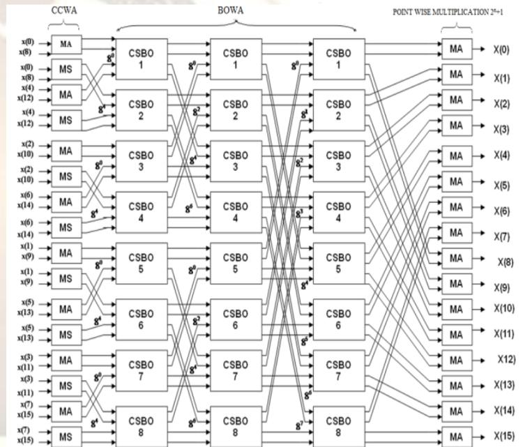
Fig.2 Internal architecture of FNT which includes ccwa, bowa and point wise multiplication  $2^n+1$
