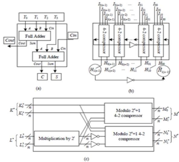
Fig. 1. Elementary operations of FNT architecture with unity root 2 (a) 4-2 compressor (b) Modulo  $2^n+1$  4-2 compressor (c) Butterfly operation without addition
