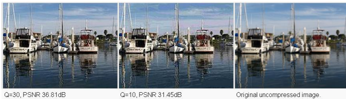
Fig.5: Example luma PSNR values for a jpeg compressed image at various quality levels
