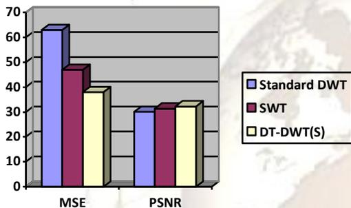
Fig.(7):MSE Vs Peak Signal-to- Noise Ratio(Soft Thresholding)
