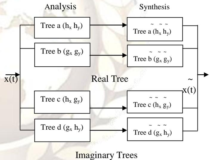
**Fig.(5) Filter bank structure for 2-D DT-DWT**
