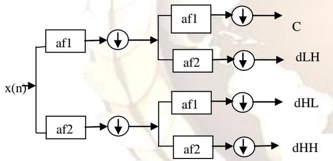
Fig.(2): One stage in multi-resolution wavelet decomposition of an image  $x(n)$
