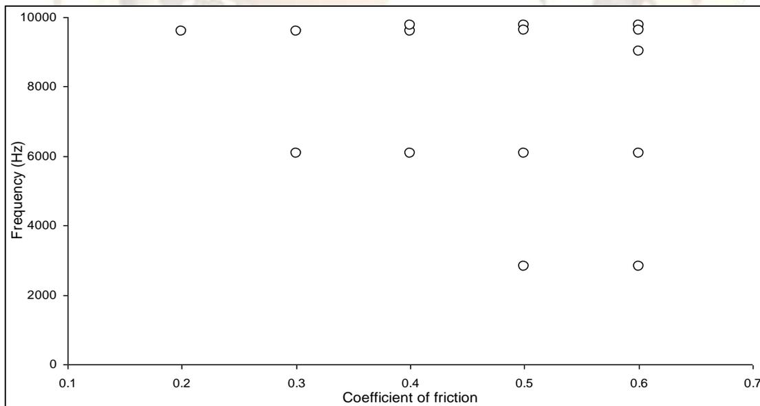
Figure 7. Prediction of unstable frequencies with variation of friction coefficient
