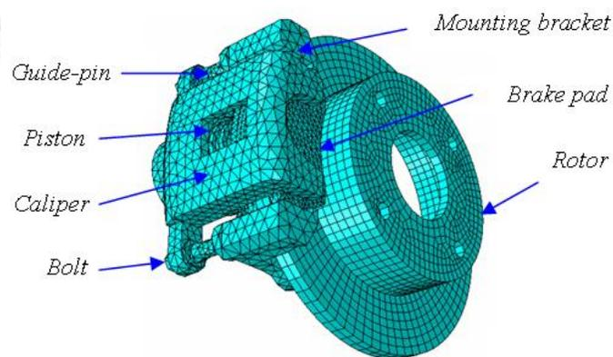
Figure 1. Finite element model of disc brake assembly
