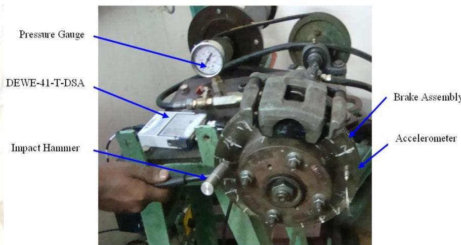
Figure 4. Experimental modal analysis of disc brake assembly.
