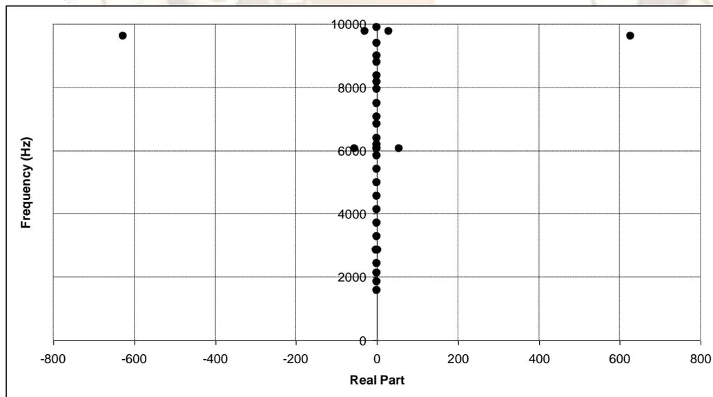
**Figure 5.** Eigenvalues extracted from the disc brake model plotted on the complex plane at  $\mu = 0.45$ .
