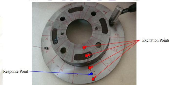
**Figure 3.** Brake rotor experimental mesh geometry.
