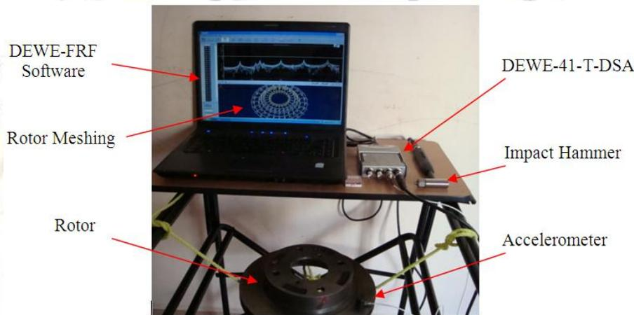
Figure 2. Experimental Modal Analysis set-up
