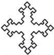
Figure1: Example of Minkowski Square Loop fractal antenna[19]
