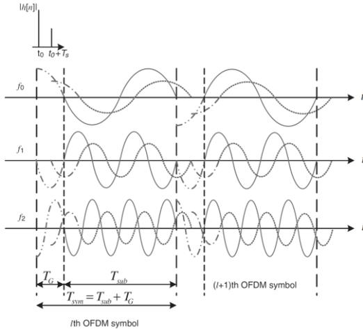
Fig. 3(b) ISI Effect of a multipath channel for each sub-carrier [4]
