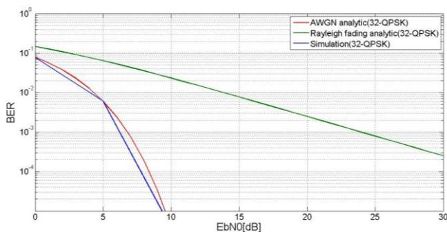
Fig. 7(c) GP length:  $N_g = N/2 = 32$  with QPSK
