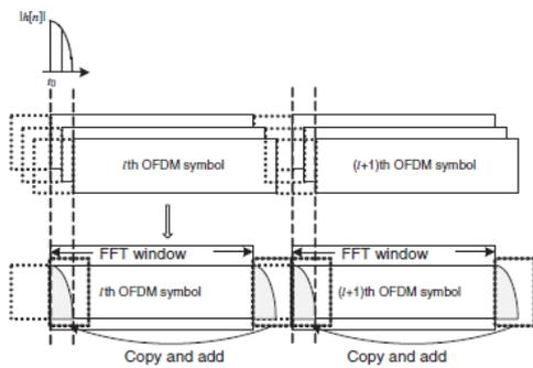
Fig.6. Copying and adding the guard interval of the next symbol into the head part of the current symbol to prevent ICI. [5]
