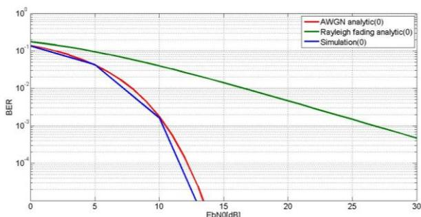
Fig. 7(d) GP length:  $N_g = 0$  (i.e. no GP) with QPSK
