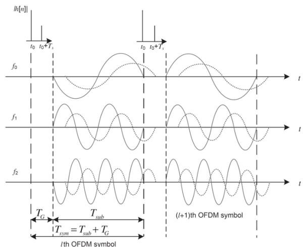
Fig. 5(b) ISI Effect of a multipath channel on OFDM symbols with ZP [4]
