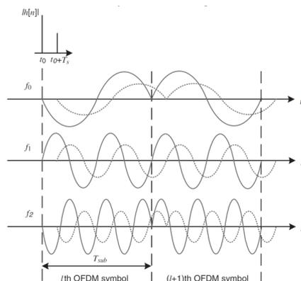
Fig. 2(b) ISI Effect of a multipath channel for each sub-carrier [4]
