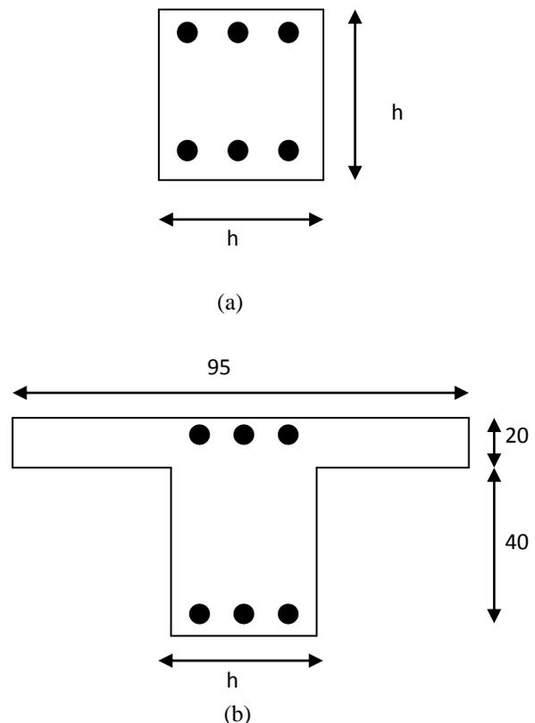
**Figure 2: Members cross section (dimensions are in cm)**
