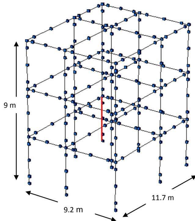
**Figure 1: The finite element model of the studied irregular building**
