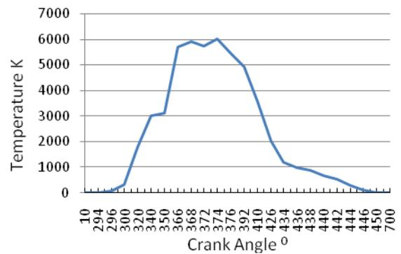
Fig. 8. Temperature V/s Crank Angle
