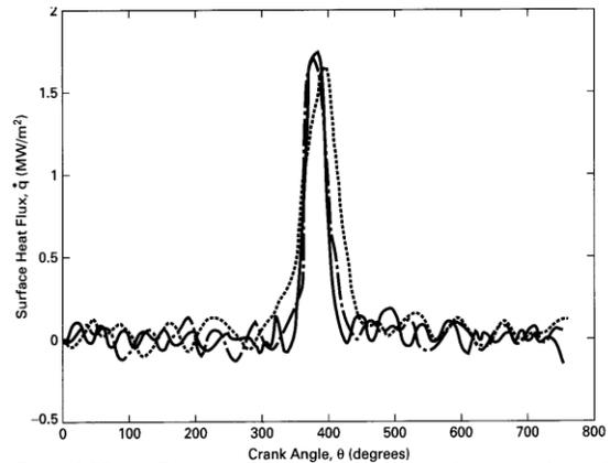
Fig. 4. Local Heat flux variation experienced at one location in a single cylinder of a typical engine for three consecutive engine cycles.
