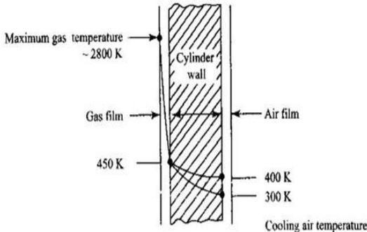
Fig. 3. Cylinder Wall Temperature Distribution of a Properly Cooled Cylinder
