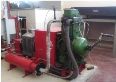
Fig. 6. Single Cylinder I.C. Engine
