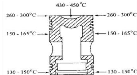
Fig. 2. Piston Temperature Distribution
