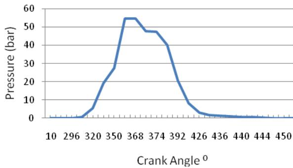
Fig. 9. Pressure V/s Crank Angle
