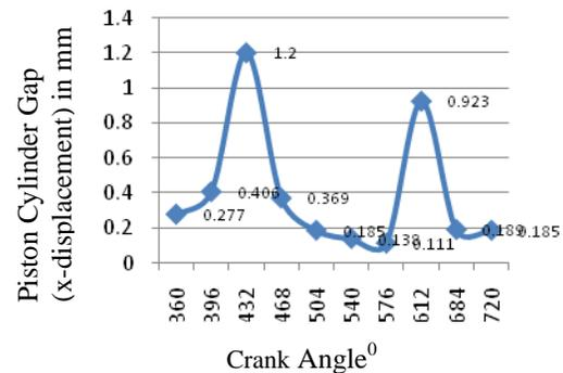
Fig.11. Variation of piston-cylinder gap for different crank angles
